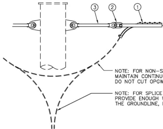
NOTE: FOR NON-SPLICE BOX LOCATIONS, MAINTAIN CONTINUOUS LOOP AND DO NOT CUT OPGW.
