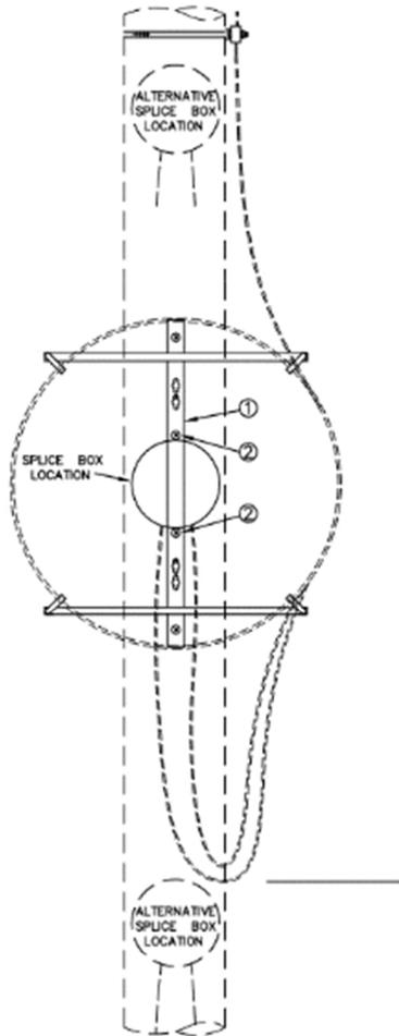
NOTE #1: ASSEMBLY WILL TYPICALLY BE Banded TO POLE USING 3/4" SS BAND MATERIAL AND ADAPTERS SUPPLIED WITH THE SPLICE BOX. ALTERNATELY, THE COIL BRACKET ASSEMBLY MAY BE SECURED WITH TWO 1/2" BOLTS (ITEM 2) USING ANY TWO OF THE FOUR THREADED RECEIVER PROVIDED.
