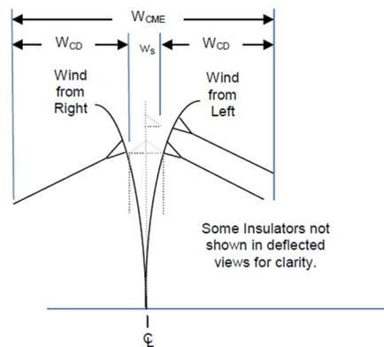
Notes:  $w_s$  = Effective Structure Width (Outboard Conductor Spacing)  $W_{CME}$  = Width, Conductor Movement Envelope;  $W_{CD}$  = Displaced Conductor Position Including Structure Deflection
